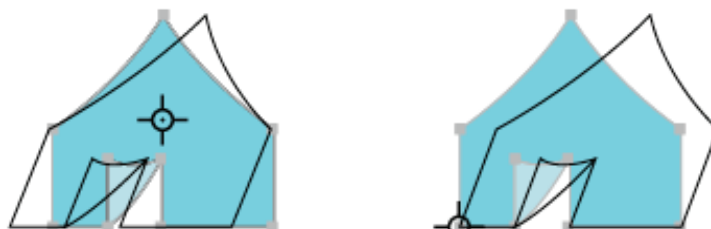
Figure 13 Shearing relative to the center (left) compared to shearing relative to a user-defined reference point (right)
